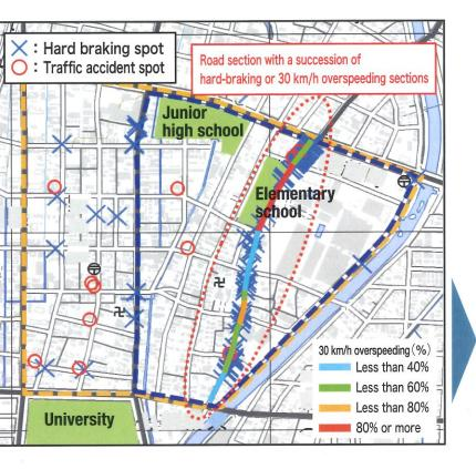
ETC2.0 is capable of collecting not only route information, but also data on details such as hard-braking spots and vehicle speed.
