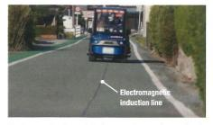
Automated vehicles recognize their positions by detecting electromagnetic induction lines laid on the road surface.
