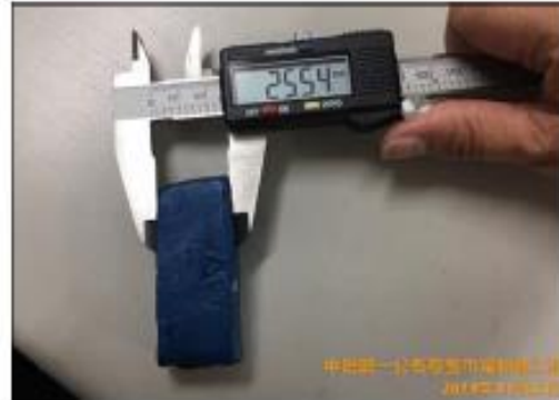
皂土條進場查驗:皂土膨脹性止水條 1"x3/4"(25.4x19.05mm) 實測:19.63x25.54mm
